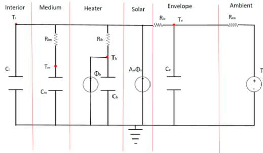
This model has six parts that will be combined in order to estimate the rest of the models. The parts are the interior, the medium, the heater, the solar radiation, the envelope and the ambient.
