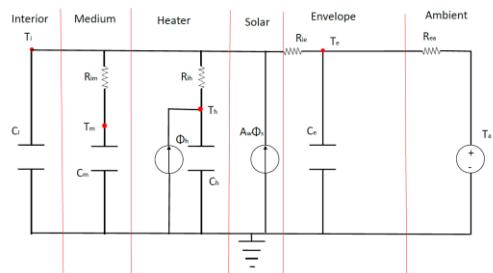
Also the heat capacities of each of the parts are presented as  $C_i$  (for the interior),  $C_m$  (for the medium part or interior wall),  $C_h$  (for the heater) and  $C_e$  (for the building envelope). Moreover, also the effective window area ( $A_w$ ) is estimated.
