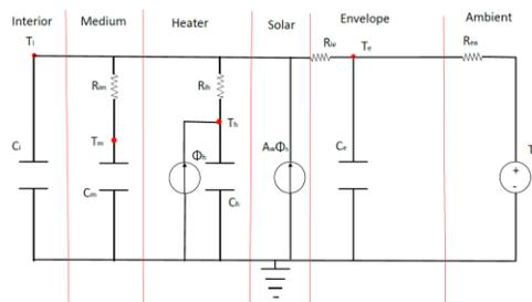
Also the heat capacities of each of the parts are presented as  $C_i$  (for the interior),  $C_m$  (for the medium part or interior wall),  $C_h$  (for the heater) and  $C_e$  (for the building envelope). Moreover, also the effective window area ( $A_w$ ) is estimated.
