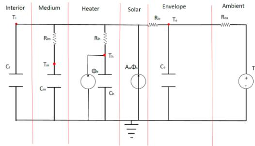
This model have six parts that will be combined in order to estimate the rest of the models. The parts are the interior, the medium, the heater, the solar radiation, the envelope and the ambient.
