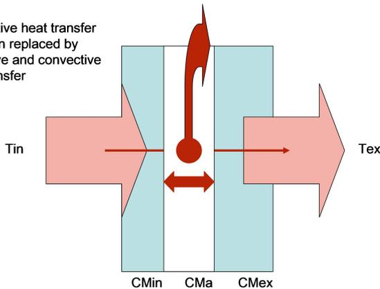
*Thermal transmission by conduction, convection and radiation*
