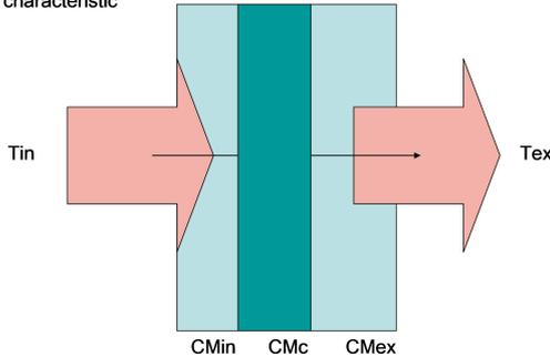
*One-dimensional thermal transmission conduction*
