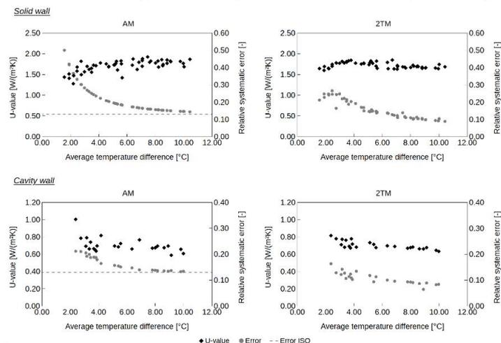
Figure 1: U-value and associated relative systematic error for the average and dynamic method (2TM model) for the solid and cavity wall as a function of the average temperature difference. The uniform error from ISO 9869-1:2014 Standard is also shown
