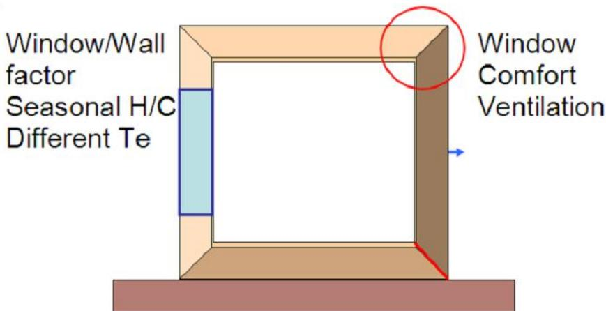
*Thermal transmission by ventilation, infiltration, conduction, convection and radiation*
