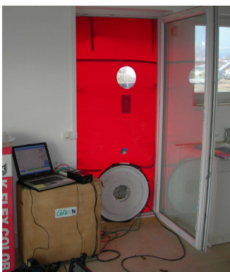
Airtightness test (blower door) in experimental houses.
