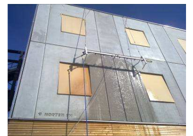
Water tightness analysis of the prefabricated concrete façade element
