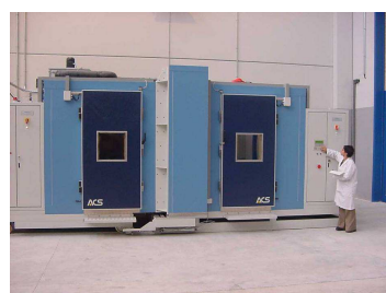
Guarded hot box for opaque walls (according to EN ISO 8990)
