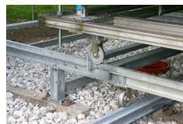
Rail system for placement of the movable Coldbox.
