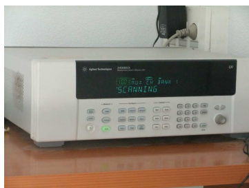
HP Agilent 34980A data acquisition system for logging and controlling the PASLINK tests.
