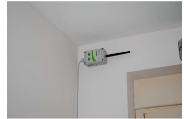
Sample sensor used for measuring temperature and humidity levels throughout the house.
