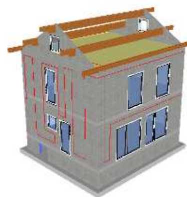
Optical fiber temperature continuous sensor.
