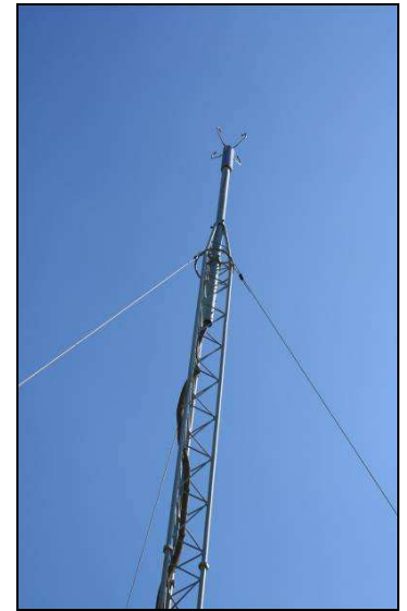
Ultrasonic device measuring wind speed and direction.
