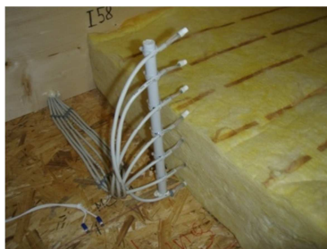
Combined heat/moisture sensors in roof assembly
