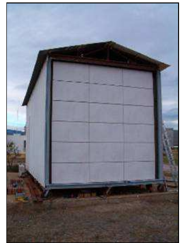
Ceramic ventilated façade being tested in a CESPA test cell.
