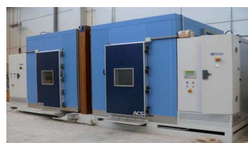
Guarded hot box for windows (according to EN ISO 12567)
