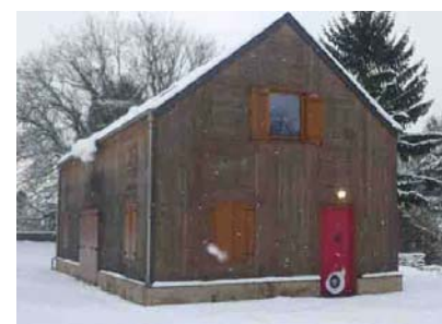
Blower-door test conducted on the building
