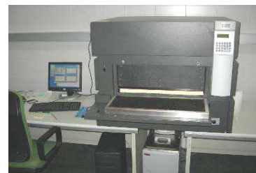
Heat flow meter apparatus (according to EN ISO 8301)
