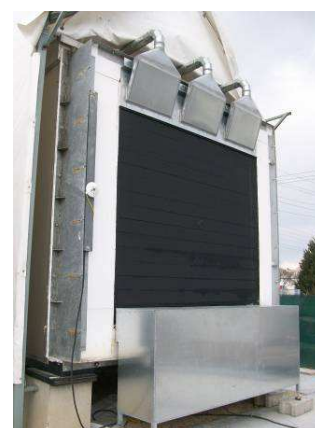
Ventilated façade with outer skin filled by PCM.
