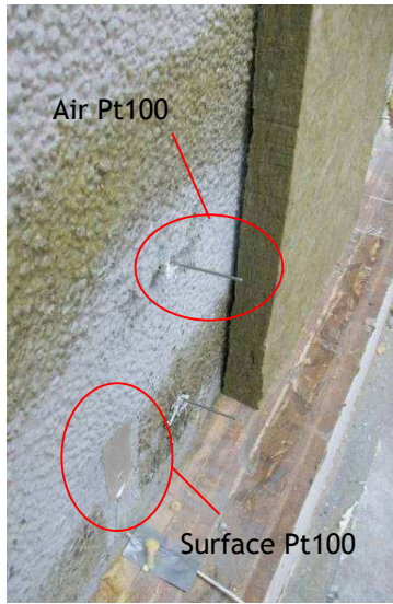
Left: Pt100 for air chamber and surface Pt100 installed below the insulation layer. Right: Distribution of air Pt100 in the air chamber.
