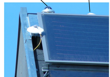
Pyranometers and pyrgeometer at the roof of EnergyFlexLab.
