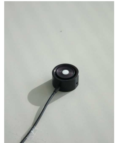
Photometer head for determining luminance (upper image) and lighting levels (lower image)
