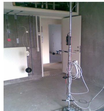
Air, globe and surface temperature sensors, humidity sensors, lux sensor and heat flux sensor in one side-by-side room in EnergyFlexLab.
