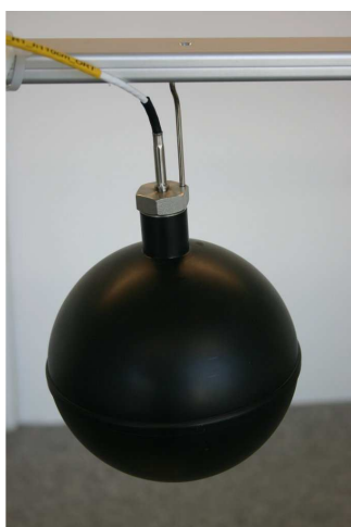
Temperature sensor for determining the operative temperature and air temperature
