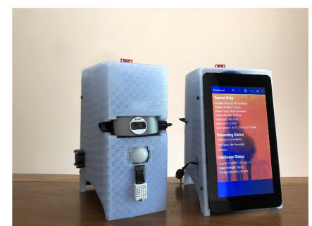
Figure 1: Our temporal thermographic sensor system, Thermporal, is designed to collect and store all the data necessary for performing quantitative analysis of insulation performance and includes: a FLIROne thermal camera, environmental sensors, and a Wi-Fi connection for accessing weather data; users primarily interact with the system using a touchscreen display.
